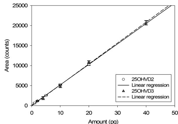
**Figure 3.** Linearity of response in the quantification of vitamin D isoforms derived from standard vitamins directly deposited on the *Collection Disc* from a plasma extraction card.
