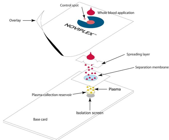
Figure 1. Illustration of the plasma extraction card.
