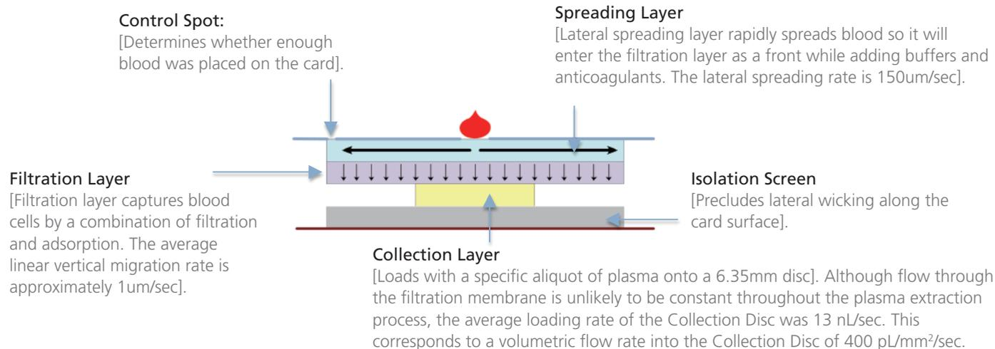
Figure 1. Noviplex plasma separation card workflow (Cont'd)
